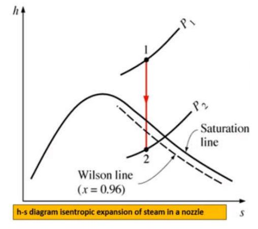
Due to high velocities, the residence time of the steam in the nozzle is small, and there may not sufficient time for the necessary heat transfer and the formation of liquid droplets.
