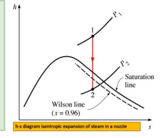
Consequently, the condensation of steam is delayed for a little while. This phenomenon is known as super saturation, and the steam that exists in the wet region without containing any liquid is known as supersaturated steam.
