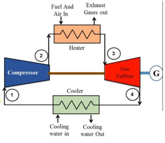
The Processes that take place in Brayton cycles. (i) Process (1-2) = Reversible adiabatic (or) I sentropic Compression (ii) Process (2-3) = Constant Pressure heat addition (iii) Brocess (3-4) = Reversible adiabatic (or) Isentropic Expansion (11) Brocess(4-1) = constant Bressure heat rejection.
