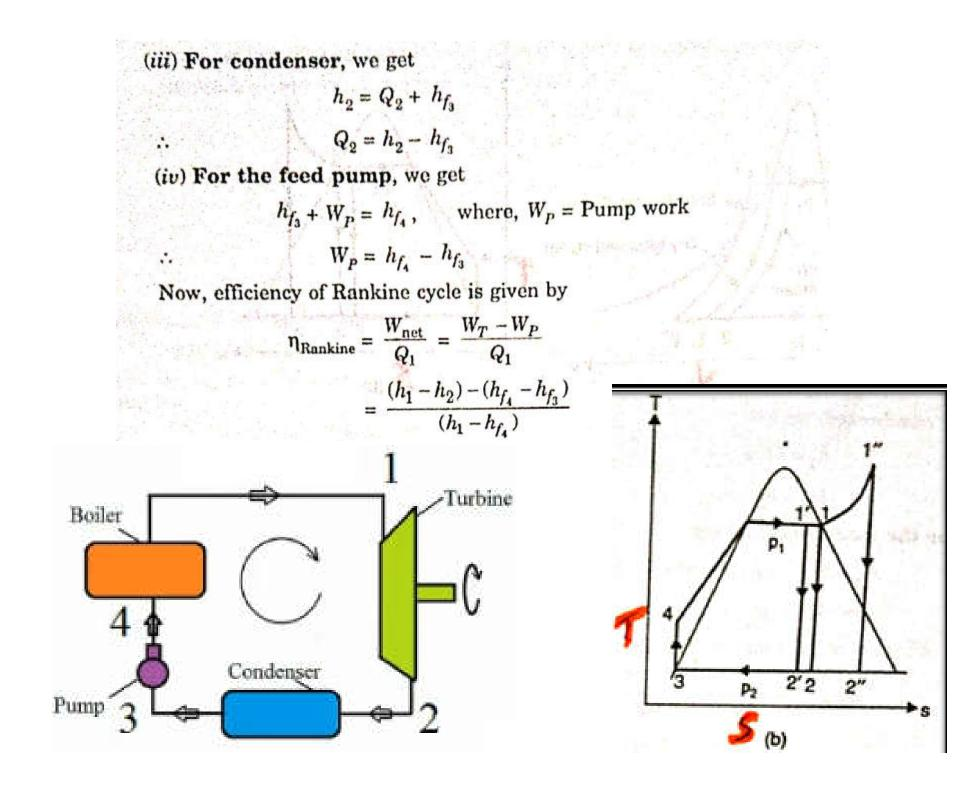
The feed pump term  $(h_{f_4} - h_{f_3})$  being a small quantity in comparison with turbine work, W<sub>T</sub> is usually neglected, especially when the boiler pressures are low.
