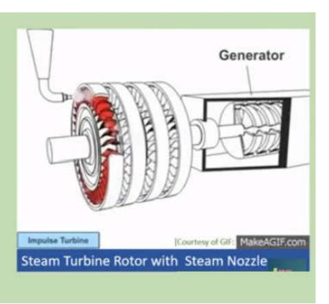
It is a passage of varying cross sectional area by means of which pressure energy of working fluid as steam is converted into kinetic energy.
