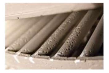
If steam quality is less than 85% Erosion of turbine blade take place Which decrease the life of turbine
