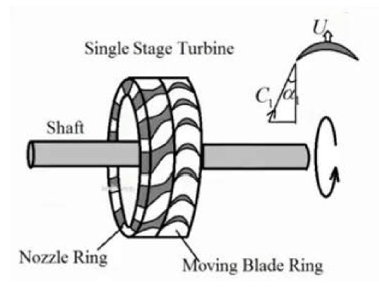
$U_{opt} = \frac{C_1 \cos \alpha_1}{2}$ in case  $\alpha_1 = 20^{\circ}$  $C_1 = 1200m/s$  $U_{opt} = 1127m/s$ In case D of Rotor is 1m then  $N = \frac{U}{\pi D} \times 60$ N = 21535 R.P.M
