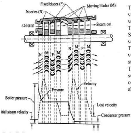
To take advantage of both pressure compounding and velocity compounding, a combination of pressure and velocity compounding is used.
