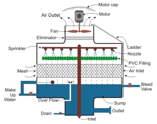
**Mesh:** When the fan is ON, it uses atmosphere air which contains some unwanted dust particles. Mesh is used to stop these particles and do not allow to enter dust in to **cooling tower**.
