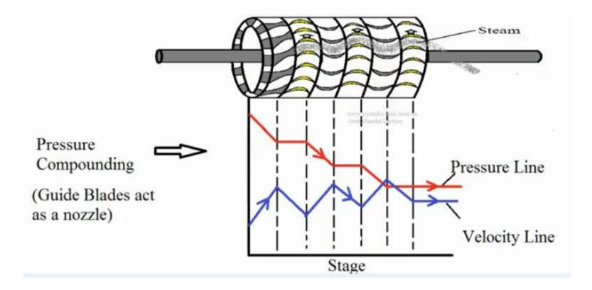
In this type of turbine, the total pressure drop (steam generator pressure to condenser pressure) is divided into number of stages.
