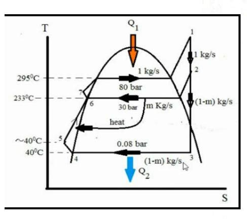
In order to find Mass flow rate (m):  $\dot{m}(h_2-h_6) = (1-m)(h_6-h_5)$ m (h2-h1) = (h6-h5) - m(16-h5) m ,-h<sub>s</sub>) = + m(h, - 4,mh 6 + m/6 - m/5 -45 m (h, -he
