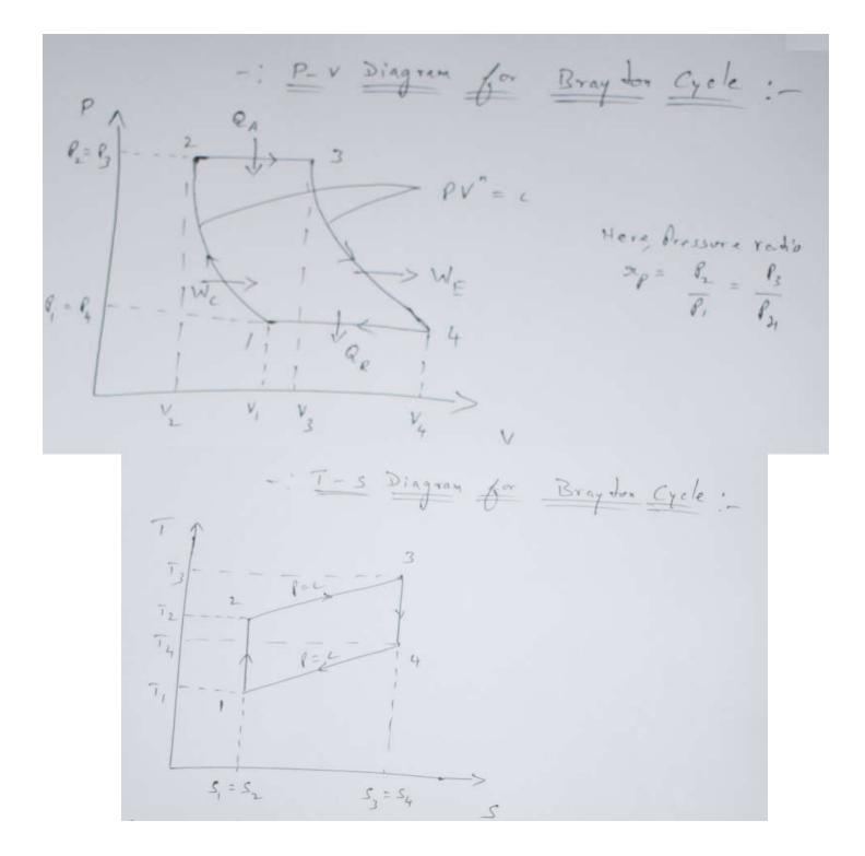
Thermal efficiency for Braydon Cycle is given by?
