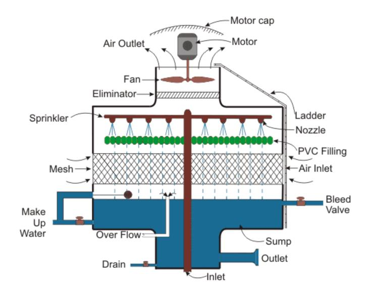
Fig. Schematic Diagram of Cooling tower
