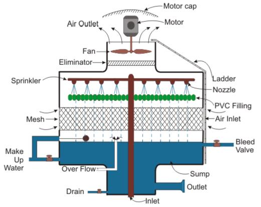
At the top the cooling tower, fans are used to lift air from bottom to the top. Because of slow speed and more contact area of water, it makes a good connection between air and hot water. The process will reduce the temperature of water by evaporation process and cooled water is collected at the bottom of the cooling tower, and this cooled water is used again in the <u>boiler</u>.
