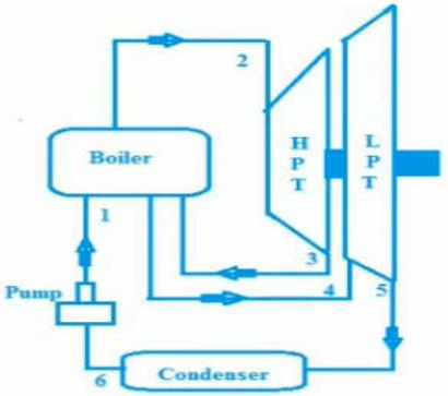
The efficiency of the simple Rankine cycle can be improved by **increasing the pressure and temperature** of the steam entering into the turbine.
